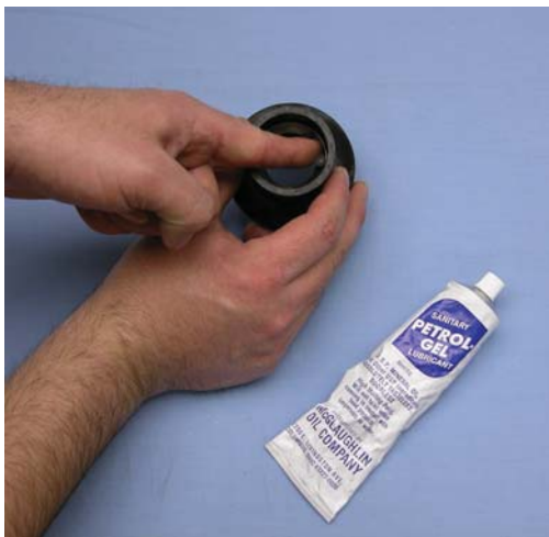
Figure 3-6 Lubricate Rear Seal
